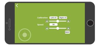
The robot's moving slow? Let's hit Speed Calibration, where you can make your robot run faster, or slower. You can also calibrate the robot's speed difference so that it runs a perfect a straight line.
