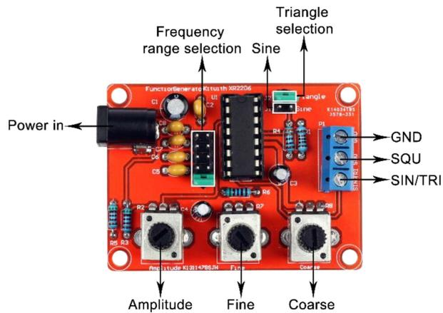
XR2206 monolithic integration function generator generates high quality, high stability, high precision sine wave, square wave and triangular wave, can realize frequency modulation and amplitude modulation, suitable for circuits such as waveform generation, Scan production, AM/FM generation, FSK generation, and a phase-locked loop.
