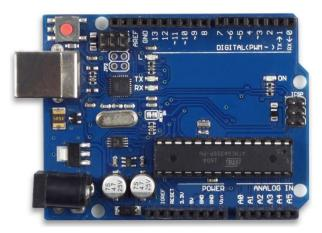
This is the new Arduino Uno R3. In addition to all the features of the previous board, the Uno now uses an ATmega16U2 instead of the 8U2 found on the Uno (or the FTDI found on previous generations). This allows for faster transfer rates and more memory. No drivers needed for Linux or Mac (.inf file for Windows is needed and included in the Arduino IDE),
