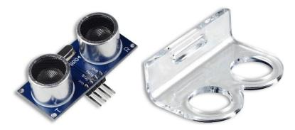
The HC-SR04 ultrasonic sensor module for Arduino is used for obstacle detection. Ultrasonic
