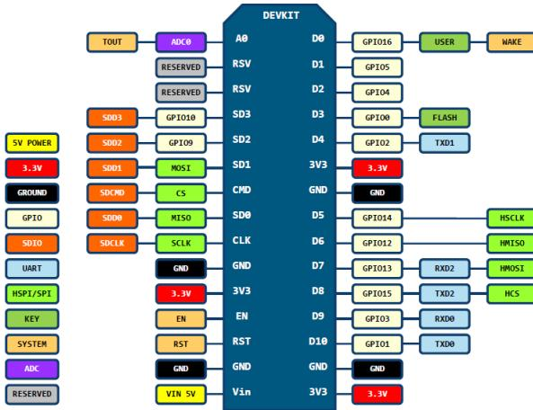
**NodeMCU DevKit Pin Map** <https://github.com/nodemcu/nodemcu-devkit-v1.0>
