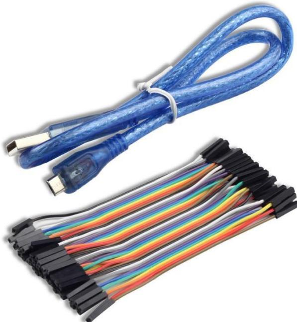
You will also need some wires to connect the display to the ESP8266. In case you want to connect the display directly to the NodeMCU you will need at least four female-to-female jumper wires, since both the display and the NodeMCU have male pin headers. The wires don't need to be long, 7.87" (20cm) is usually enough.
