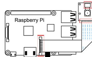
Make sure the ribbon cable is attached to the CSI port near the headphone jack instead of the DSI port on edge.
