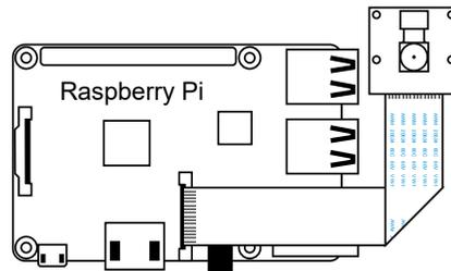
You need to connect the camera module to the Raspberry Pi's camera port, then start up the Pi and ensure the software is enabled.
