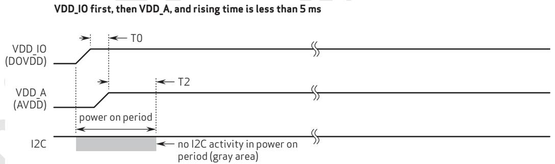
**note**  $T0 \geq 0$  ms: delay from VDD\_IO stable to VDD\_A stable
