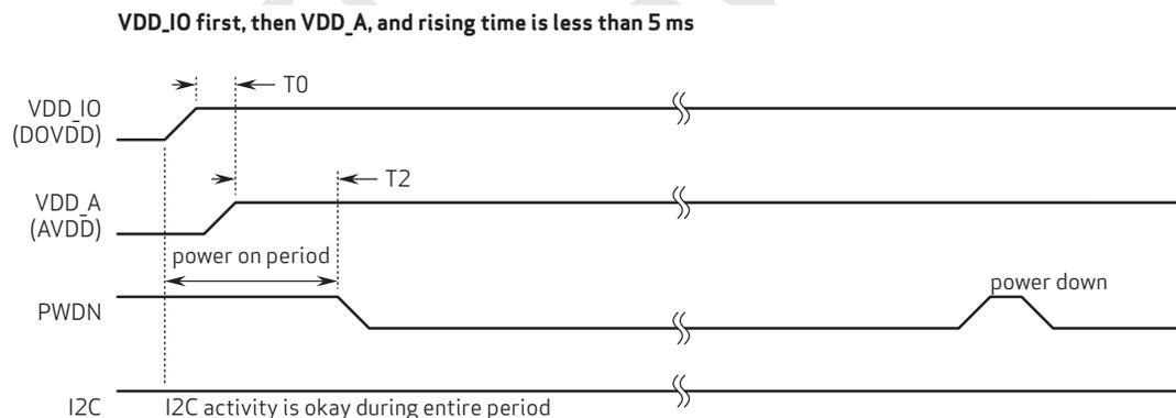
**note**  $T_0 \geq 0$  ms: delay from VDD\_IO stable to VDD\_A stable
