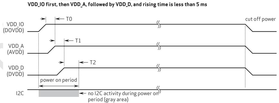
**note** T0 ≥ 0 ms: delay from VDD\_IO stable to VDD\_A stable
