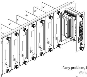
2. Insert the installed module directly, and then secure the additional captive loose-off screws in the holes on its mounting frame.
