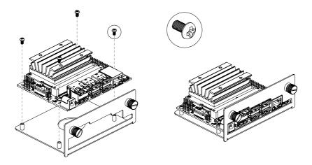
1. Attach the Jetson Nano Board to the mounting bracket with M2.5\*5 screws.
