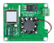
**UCTRONICS U6102** POE HAT for Raspberry Pi is to use with the Raspberry Pi models with PoE pins like Raspberry Pi 3 Model B+ and Raspberry Pi 4 Model B, so you can power the Raspberry Pi with an single Ethernet cable plugged in.
