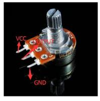
Potentiometers, sometimes called pots, are relatively simple devices. One terminal of the potentiometer is connected to a power source, and another is hooked up to a ground — a
