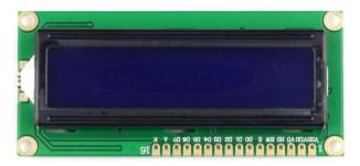
LCD1602 is a kind of character LCD display. The LCD has a parallel interface, meaning that the microcontroller has to manipulate several interface pins at once to control the display. The interface consists of the following pins:
