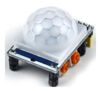
Generally speaking, motion sensor is made of thermoelectric sensor, and it can detect body motion. The motion sensor module generally uses the BISS0001 ("Micro Power PIR Motion Detector IC") to convert the analog signal from the sensor to digital output.
