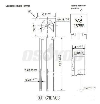
The application of the IR receiver is in project 20 (Use Raspberry pi to get IR remote code), please check the project 20 for your reference.
