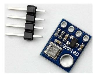
The BMP180 is the function compatible successor of the BMP085, a new generation of high precision digital pressure sensors for consumer applications.
