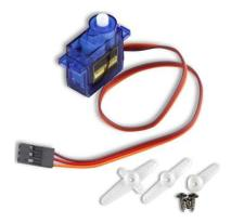
Servo is a type of geared motor that can only rotate 180 degrees. It is controlled by sending pulses signal from your microcontroller. These pulses tell the servo what position it should move to.
