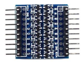
Specification of the 8 channel logic level converter
