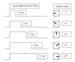
In this project (Drive Servo Motor with Raspberry Pi), we will use Raspberry Pi to send command through GPIO to Servo Motor and control its rotation action.
