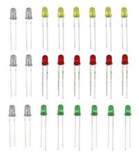
The LED is the abbreviation of light emitting diode. It is usually made of gallium arsenide, gallium phosphide semiconductor materials. The LED has two electrodes, a positive electrode and a negative electrode, it will light only when a forward current pass, and it can be red, blue, green or yellow light, etc. The color of light depends on the materials it was made.
