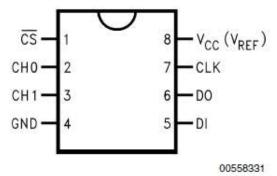
COM internally connected to GND. V<sub>REF</sub> internally connected to V<sub>CC</sub>.
